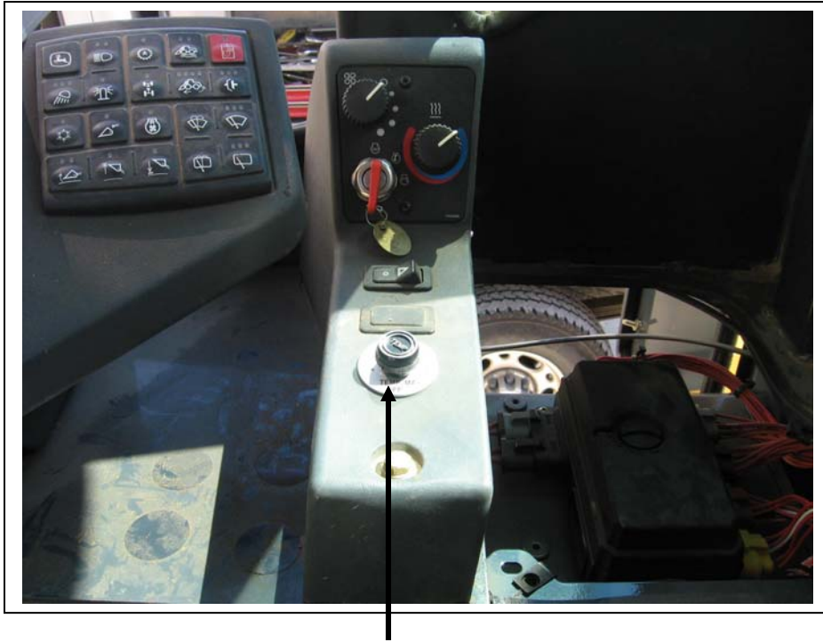
Thermostat installed near blower controls.
